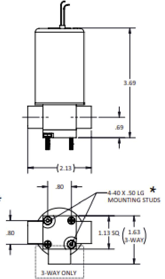
\*Two Mounting Studs are supplied. Contact us for alternate mounting options. Limit applied torque on mounting studs to 7 - 9 in-lbs max.
