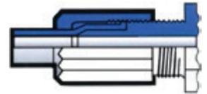
**Compression Tube:** This fitting accepts straight tube with ferrule & nut (with/without gripper). Tube fittings are the most common connection for plastic applications. They accommodate fast assembly. Nut can include an integral gripper or external gripper.
